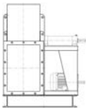
Transmission drive, identical to SYSTEM 1, with the motor and fan mounted on the common bench. Motor positions "W" or "Z" and exceptionally "X" or "Y".
