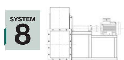
Elastic coupling drive, impeller mounted on the support shaft, mounted on the motor via an elastic coupling. Everything mounted together on a fan pedestal.
